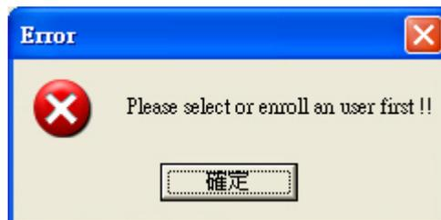
You can click the **Verify** by mouse or press the **ALT+V** by keyboard to enter the matching fingerprint mode. Before clicking the **Verify** button, you must first select a user. Otherwise the following screen will appear.
